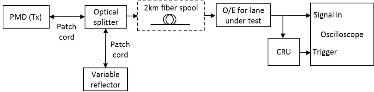
Figure 2: TDEC conformance test setup
