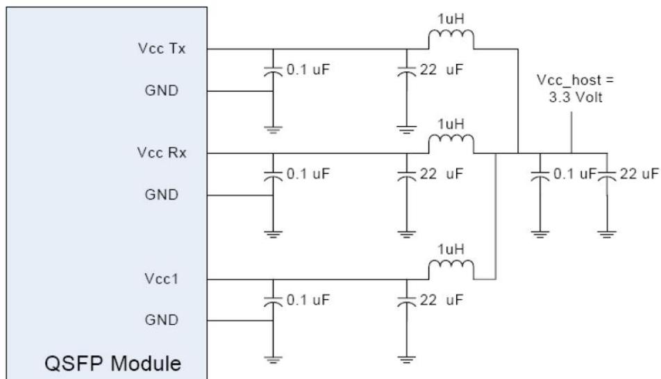
Figure 2. QSFP voltage supply and filtering scheme
