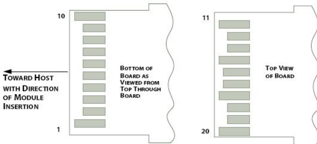
Figure 2: Module Contact Assignment
