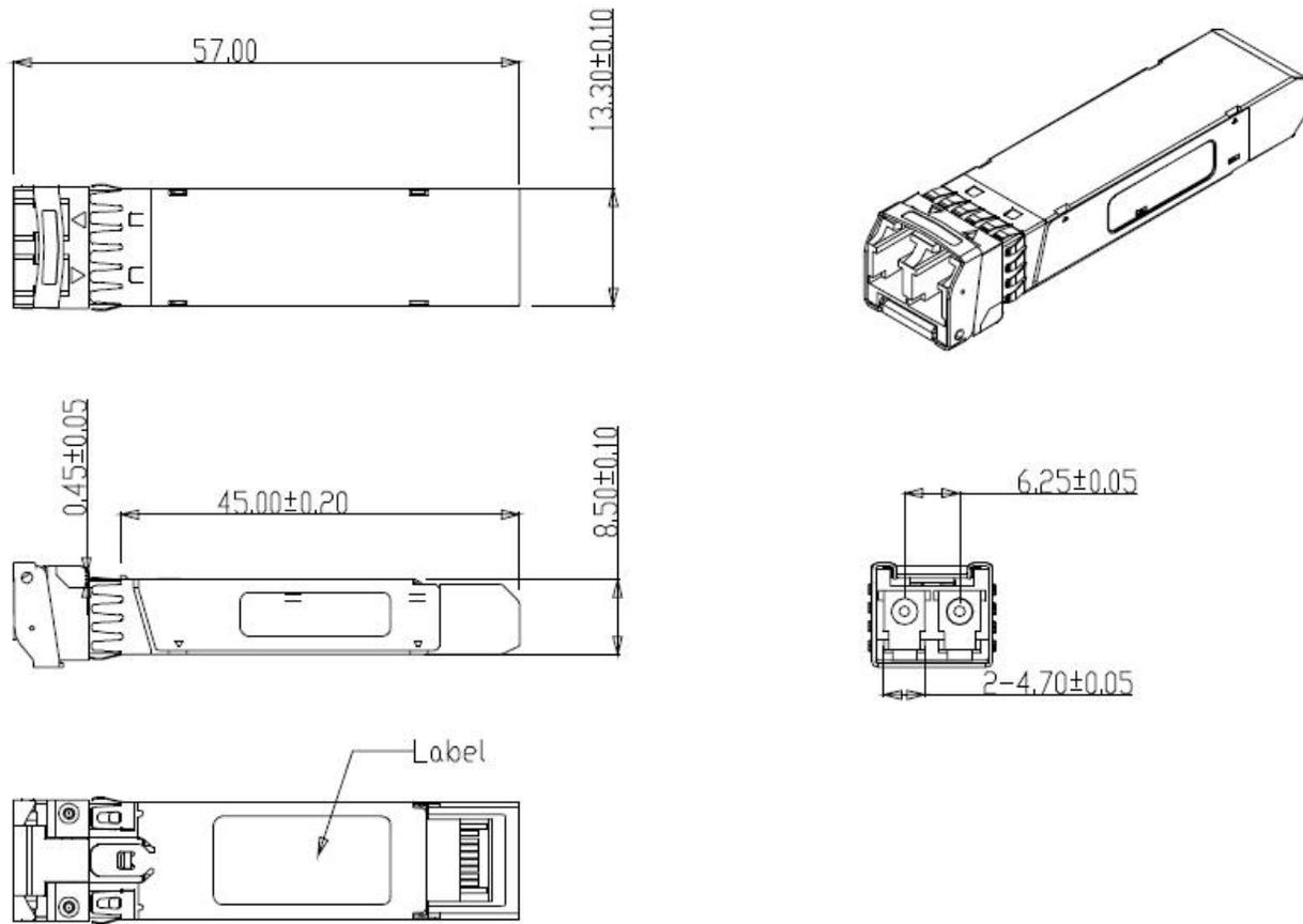
**Figure5. Mechanical Specifications**
