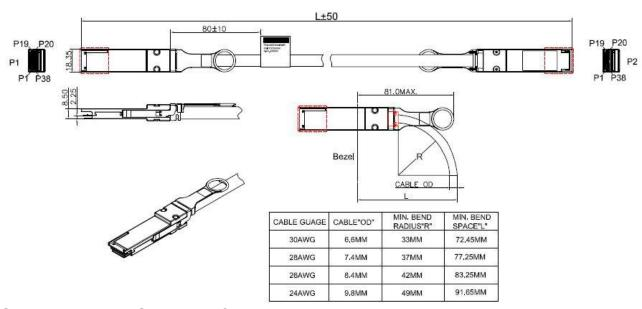
**QSFP+ Host Board Schematic for passive copper cables**
