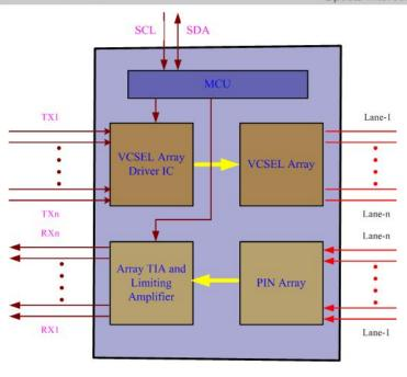
Figure 1. Module Block Diagram
