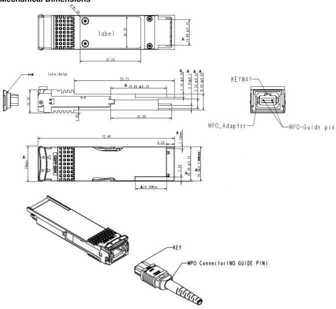
Figure 10. Mechanical Specifications
