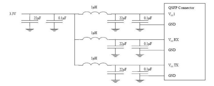
Figure 3. Host Board Power Supply Filtering
