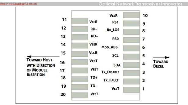
Figure2. Host PCB SFP+ pad assignment top view
