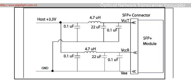
Figure 4. Host Board Power Supply Filters Circuit
