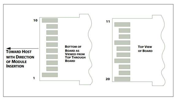
Figure3. SFP+ module contact assignment
