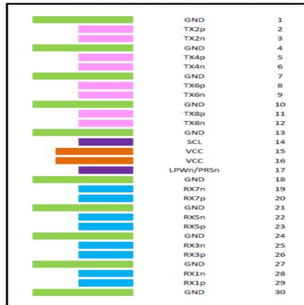
Figure3. OSFP module Pin-out Details
