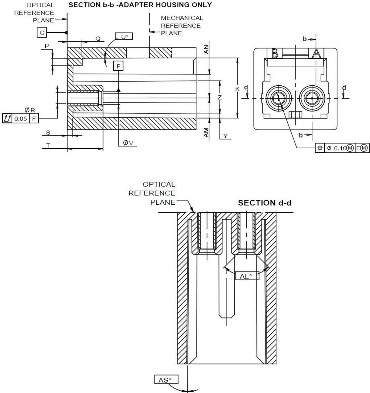
Figure 2.2.1a– Duplex adapter individual component dimensions
