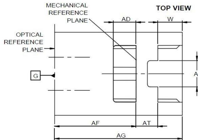
Figure 2.2.1a– Duplex adapter individual component dimensions
