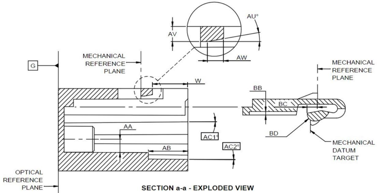
Figure 4.2a – Duplex receptacle interface
