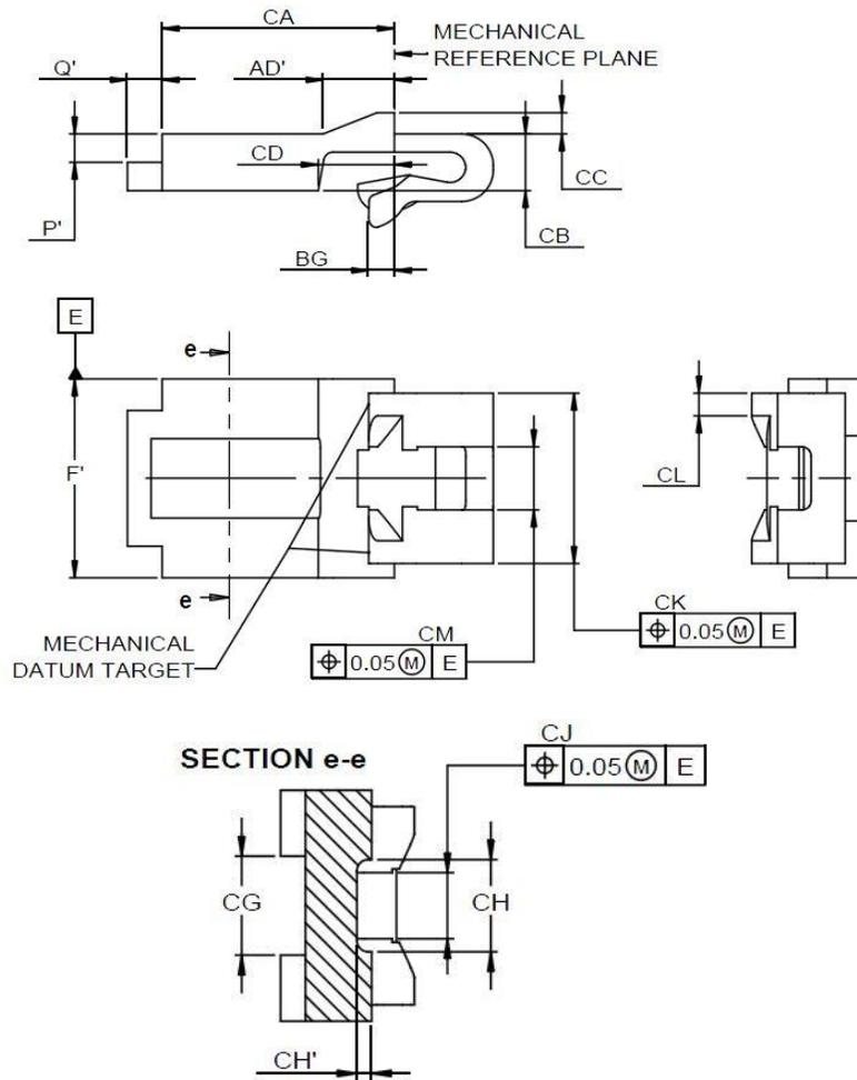
Figure 4.2a – Duplex receptacle interface, individual components dimensions
