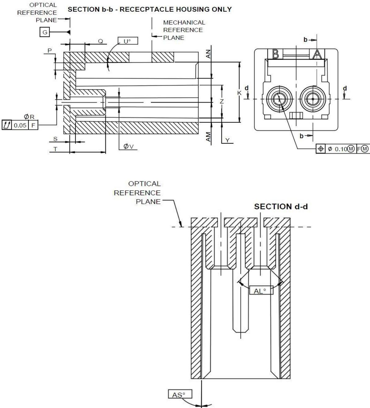
Figure 4.2a – Duplex receptacle interface
