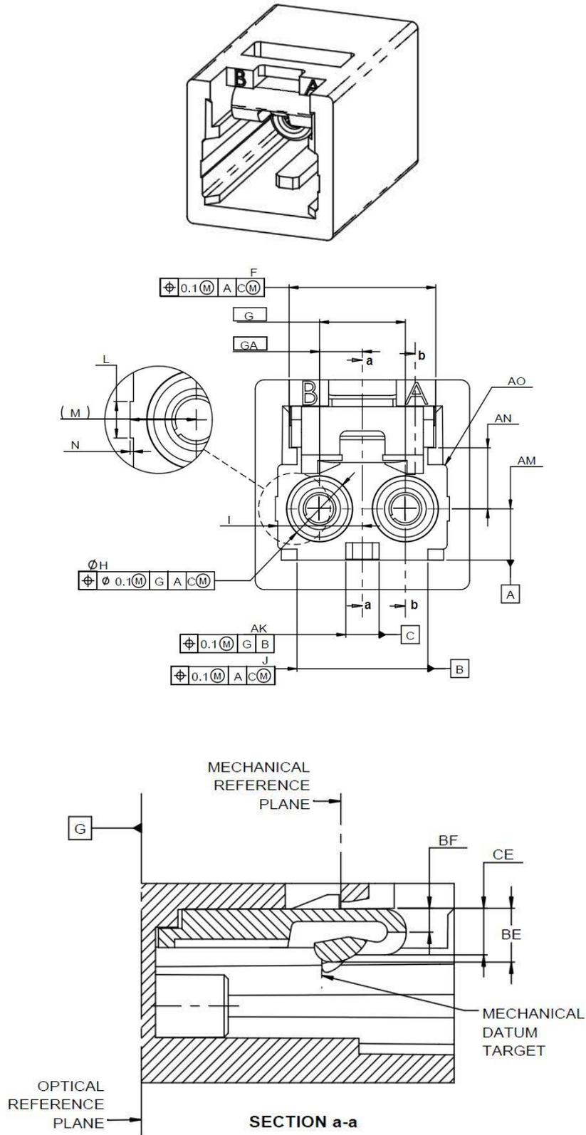
Figure 4.2a – Duplex receptacle interface
