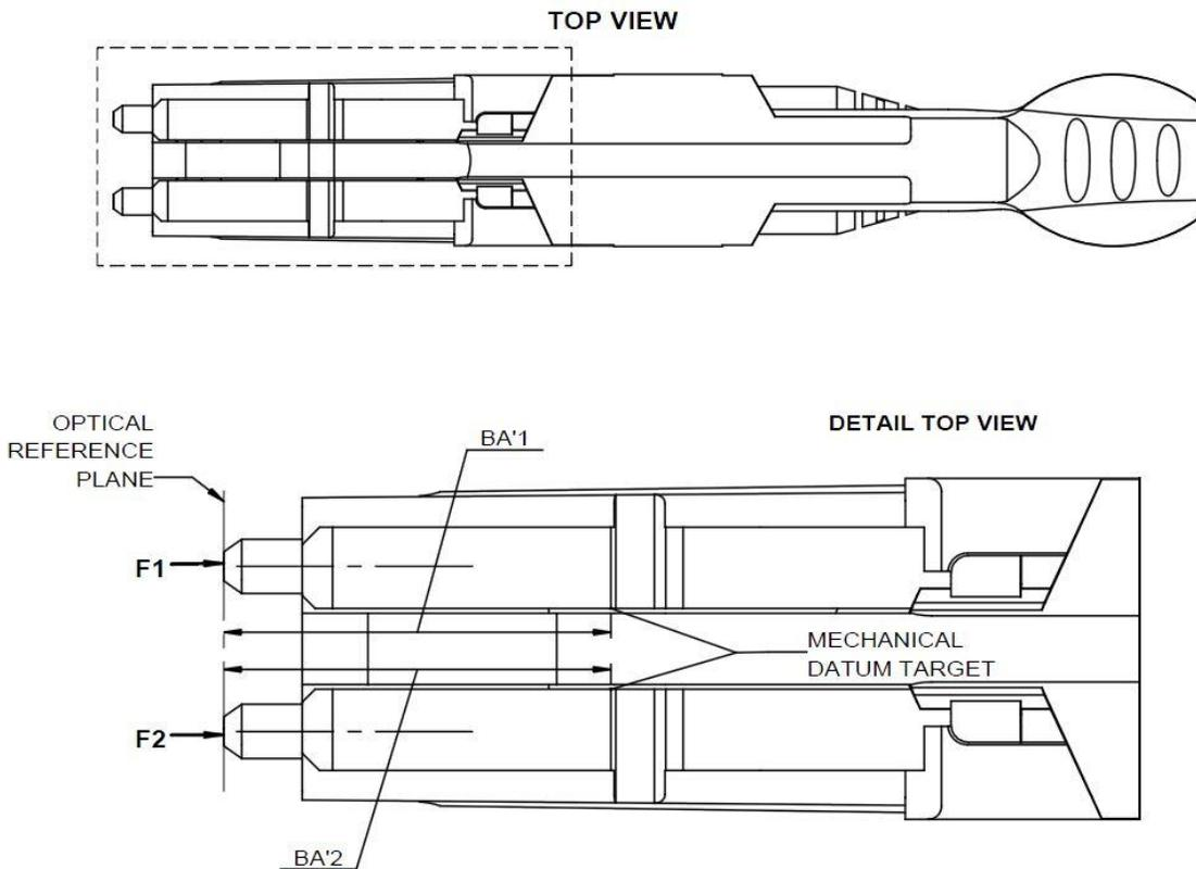
Figure 3.2.6 - Ferrule extension and contact force
