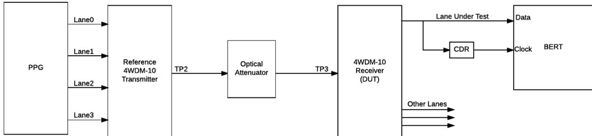
**Figure 3-1: Test setup for measurement of receiver sensitivity**
