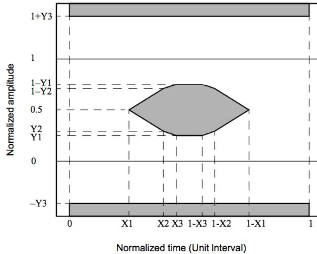
**Figure 2: Transmit Eye Mask**
