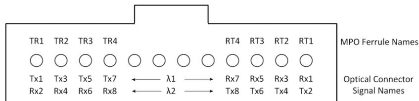
Figure 3-1: 400G-BD4.2 Lane Ordering for MPO Optical Connector
