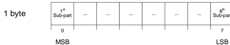
Figure 31D: 1-byte bitmask format
