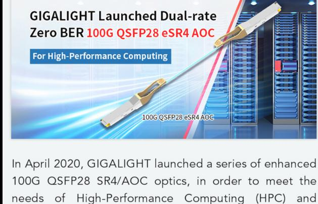
new products support 25G/28G per channel and use OM4 fiber to achieve Zero BER transmission at 100 meters without FEC. While FEC is turned on, the transmission distance can reach up to 300 meters (OM4). In addition, the industrial temperature range feature is optional. For the purpose of market segmentation, GIGALIGHT has defined and developed a series of differentiated AOC products, including the low-cost overclocking AOC lite version, the standard SR4 AOC version, the 25GE ze-
