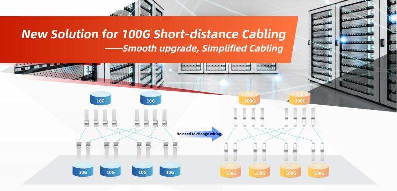
Compared with the traditional 100G short-distance transceivers based on MPO multi-fiber cabling, the two new products adopt duplex-fiber cabling. When the network architecture is upgraded from 1G/10G to 100G, by using the duplex-fiber 100G transceivers, the deployed LC duplex cabling infrastructure can be reused and additional MPO cabling is not required, saving much cabling cost. So, that the duplex-fiber 100G transceivers come to be a new choice for data center cabling.
